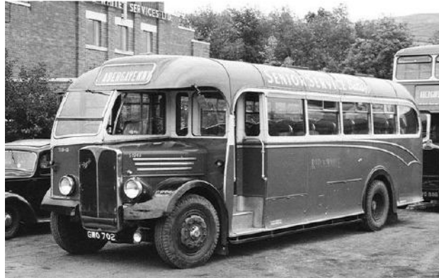
ex-Ralph's Garages 1948 Regal 9621A GWO 702 ($1949) also with standard Duple bus bodywork showing detail differences from the previous years' model.
