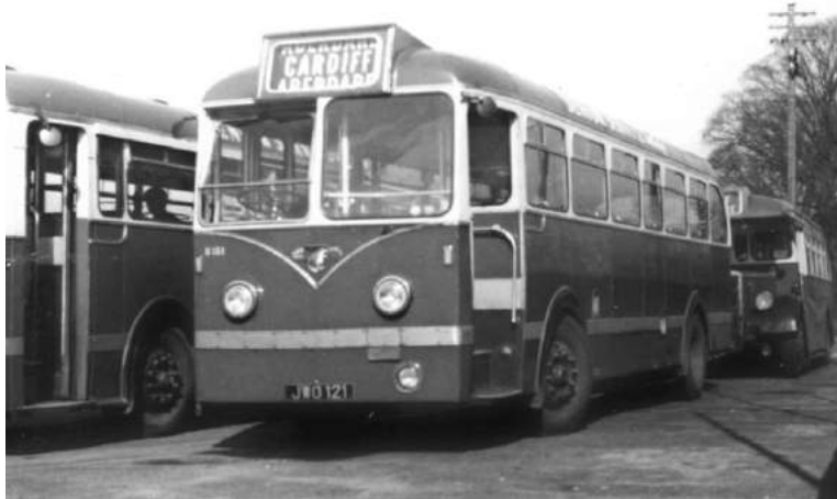
The first Royal Tiger JWO 121 (UC151) with Jicwood-designed all-alloy bodywork built by Lydney Coachworks.
