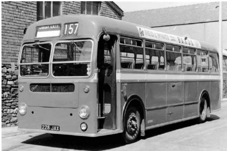
The second MW to be built was retained by Bristol as a test vehicle and was fitted with a B45F body and sold to Red & White in 1963 as 228 JAX (U1563). This had a different style destination box and side trim from the other Red & White MWs.
