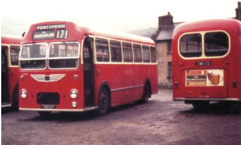
A pair of 1958 MW6Gs showing the upright rear of TWO 72 in contrast to the more rounded rear of the later MWs.
