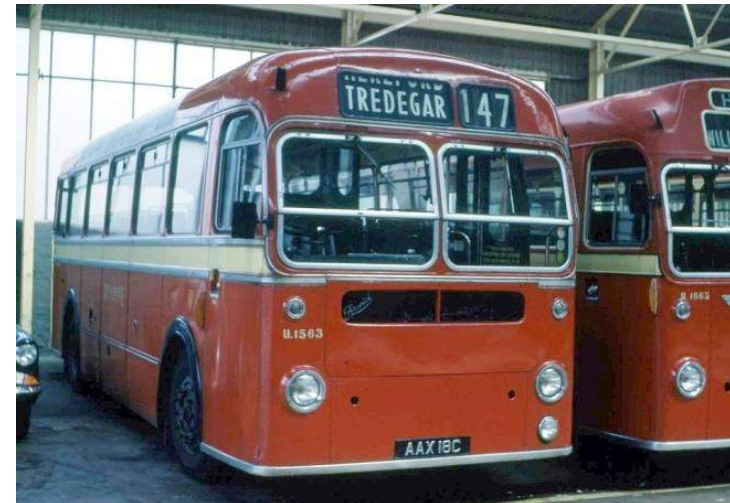
AAX 18C (U1563) at Tredegar after being rebodged with the body from withdrawn 228 JAX. (Andrew Mann)
