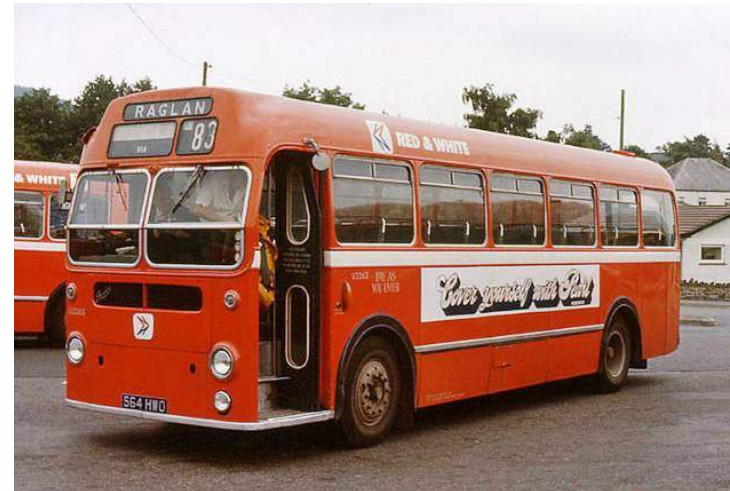
MW6G 564 HWO (U263) at Abergavenny on 13 th July 1977 in NBC livery with the later blue and red logo on a white background. It was renumbered U3663 in 1975. This batch had the Cave-Brown-Cave heating system with the radiator grille just below the windscreen. (Mike Street)
