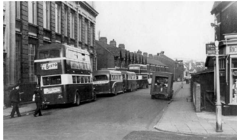
St Vincent Road, Newport ca 1952 showing Leyland Titan MV 1376 (H140) with rebodied East Lancs coachwork behind A.E.C.Regal TG5505 or TG5506, a Bedford OWB and a 1949/50 Guy Arab. (Mike Taylor)
