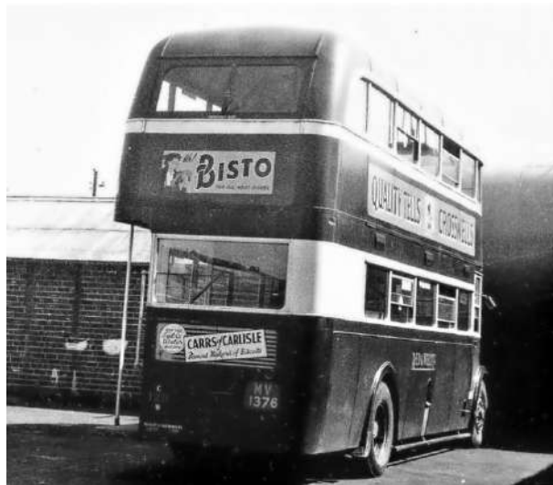
Front and rear views of Leyland Titan TD2 MV 1376 after rebodding with a second-hand East Lancs H30/26R body.
