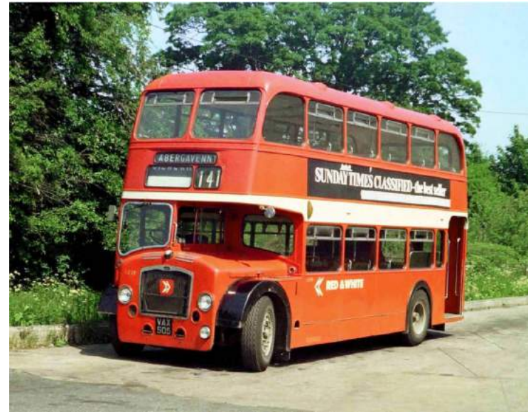
1959 Bristol LD6G VAX 505 (L559) in NBC livery and with hopper window vents. (Martin Bott)
