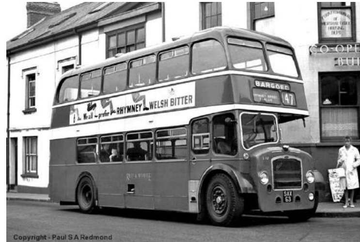
SAX 63 (L157) with shallower radiator grille, narrower destination indicator, sloping top edge to cab windows and straight bottom edge to cab door window (Paul S A Redmond)
