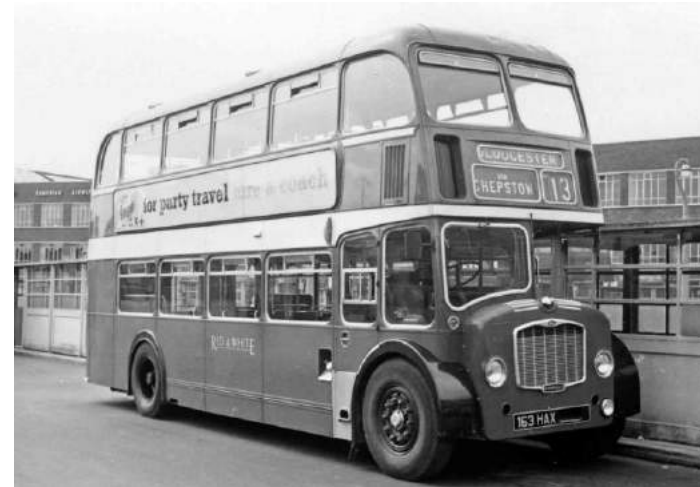
1963 Bristol FS6B 163 HAX (L163) with Cave-Brown-Cave heating and ventilating system and illuminated advertising panel at Cardiff Bus Station.
