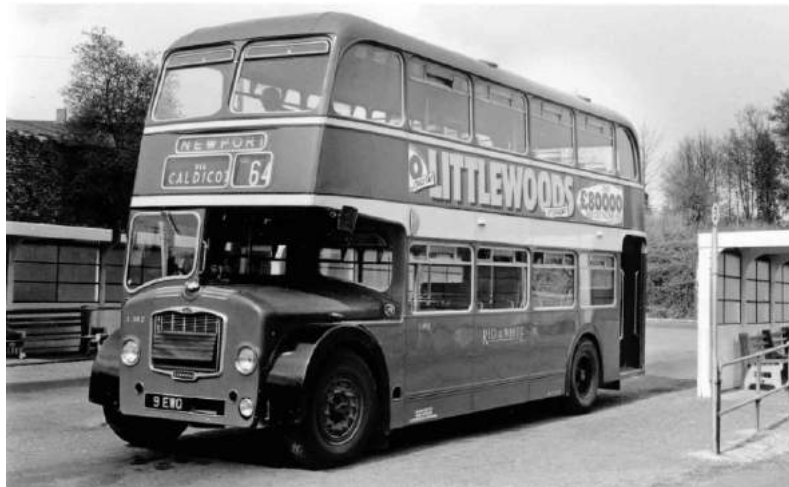
1962 Bristol FS6B 9 EWO (L962) with new style radiator grille at Chepstow Bus Station. (S J Butler Collection)
